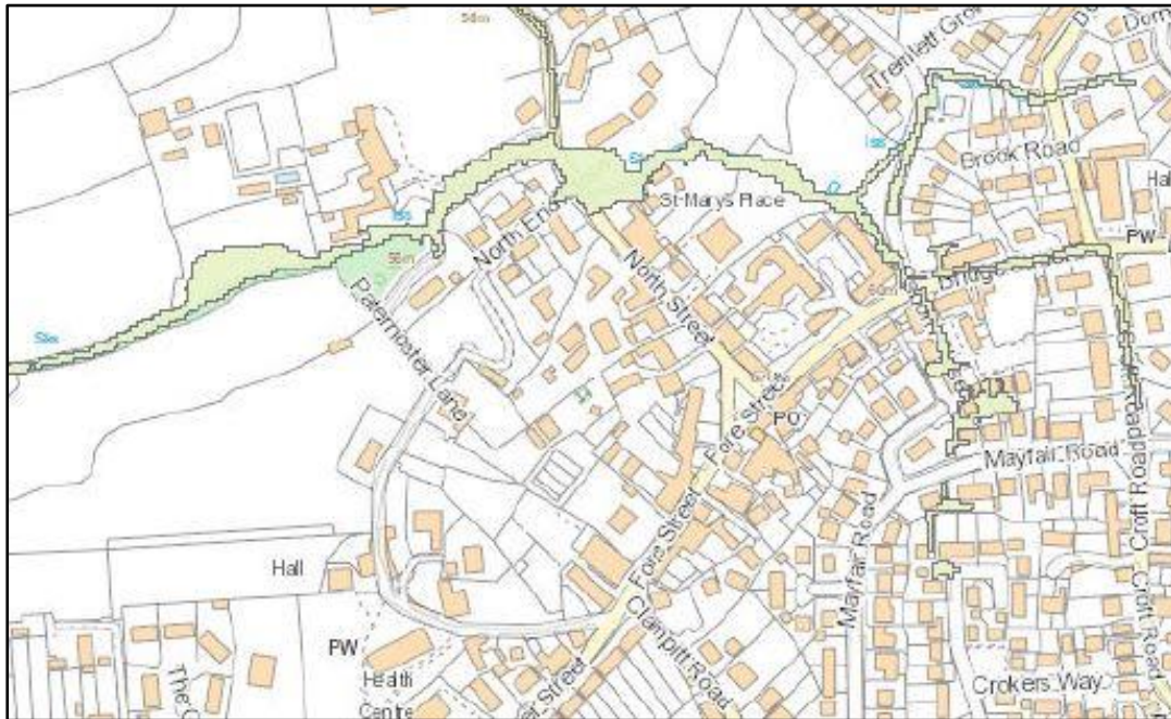
Figure 18: 1 in 30 year surface water flooding in Ipplepen Village
