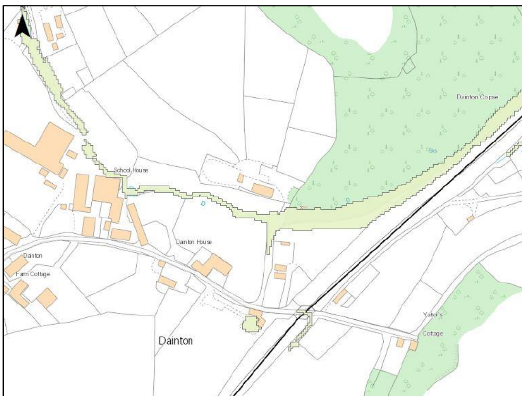
Figure 19: 1 in 30 year surface water flooding in Dainton Village
